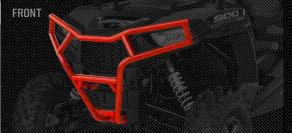
1½" DIAMETER STEEL TUBE CONSTRUCTION
